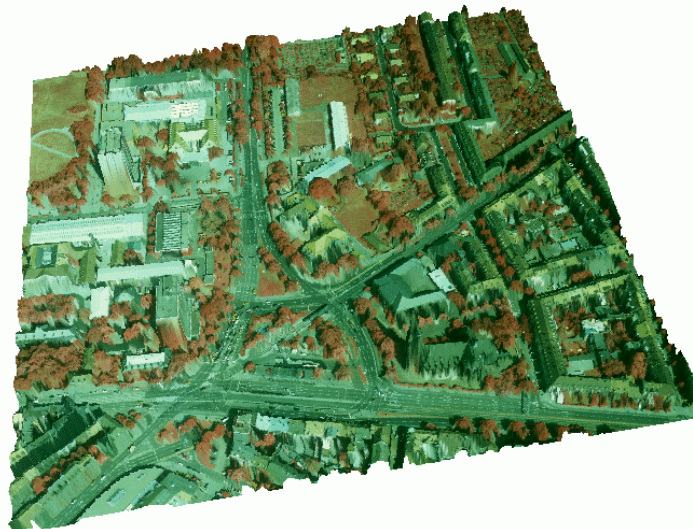
Figure 1: 3D visualization of laser DSM overlaid with CIR ortho image
