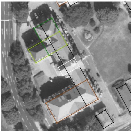
Figure 2: Ground plan decomposed into rectangles
