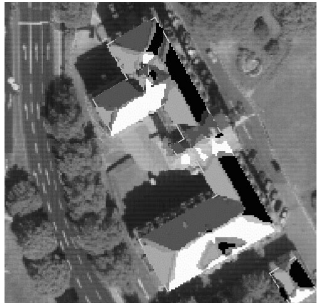
Figure 5: Segmented roof regions.
