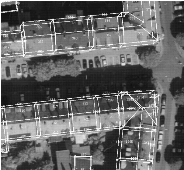
Figure 15: Reconstructed buildings projected into stereo image.
