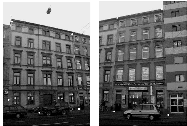
Figure 16: Original terrestrial images with points measured for rectification.
