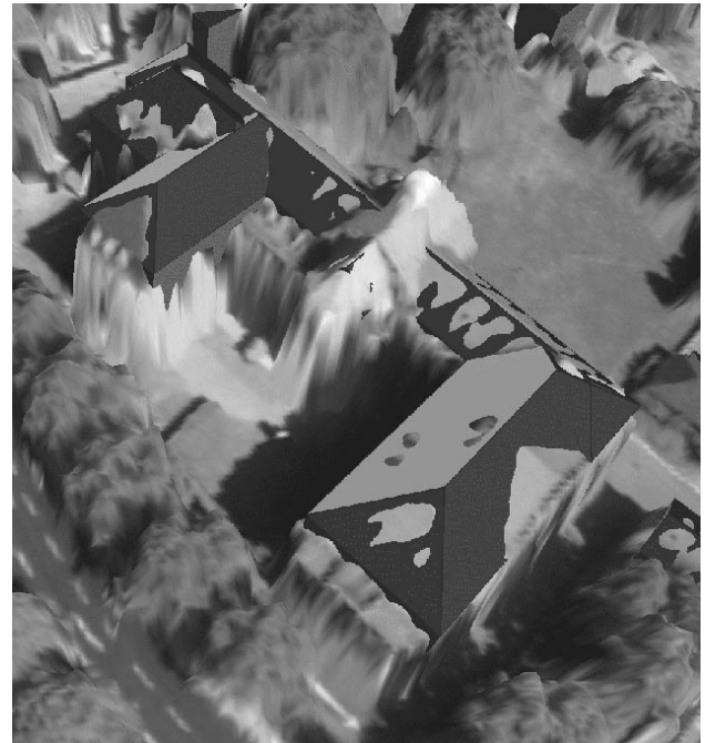
Figure 8: Reconstructed building and DSM surface.
