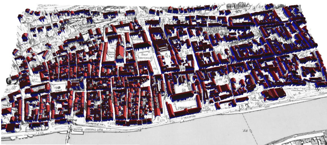
Figure 7: Automatically reconstructed buildings (city of Heidelberg) on top of DGK5 map.
