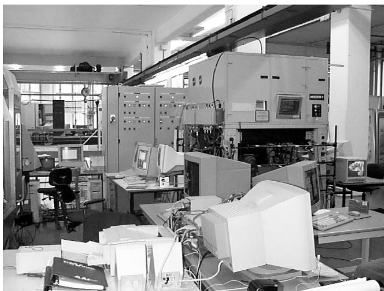
Figure 1. View of the experimental measuring platform during a test run. Foreground: several general purpose computers used for sensor specific processing, image processing, system and machine control. Background: control cabinet (left) and measuring platform (right).
