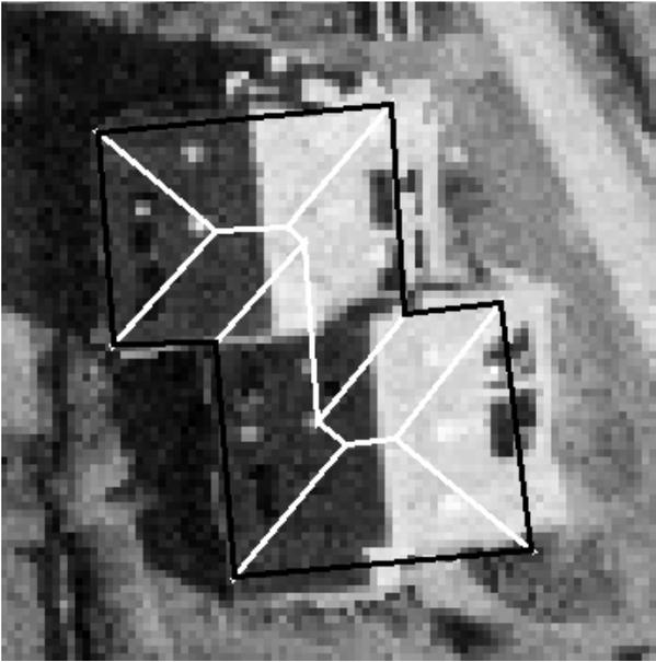
Figure 10: Given ground plan (black) and initial reconstruction (white), projected to ortho image
