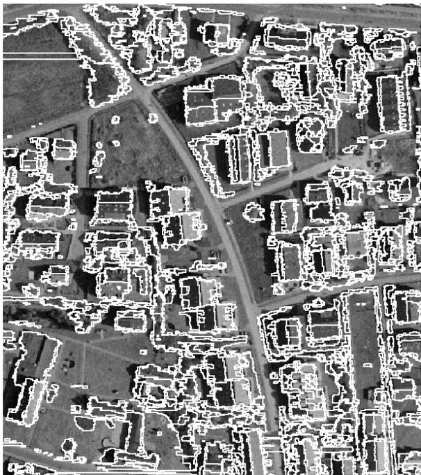
Figure 2: Planar segmentation for laser scanner DSM (overview), projected to ortho image
