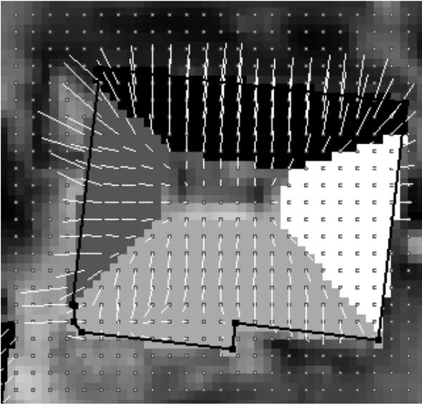
Figure 4: Building ground plan (black), DSM surface normals (white) and segmented planar surfaces
