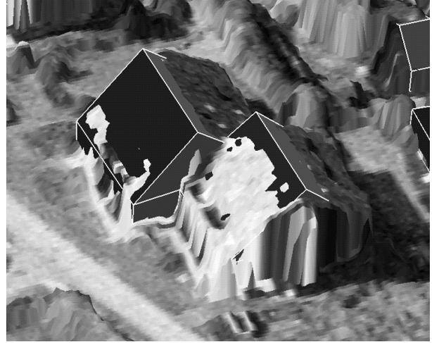
Figure 13: Adjusted reconstruction, projected to DSM.
