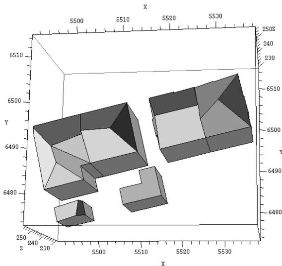
Figure 8: Reconstructed buildings, adjoining eaves lines forced to be collinear
