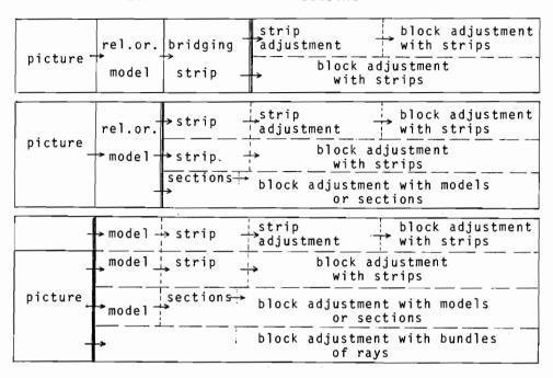
Figure 1: Schematic Diagram of the Methods of Aerialtriangulation
