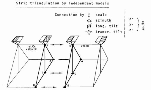
Figure 2: Schematic Diagram of the Connection of Independent
