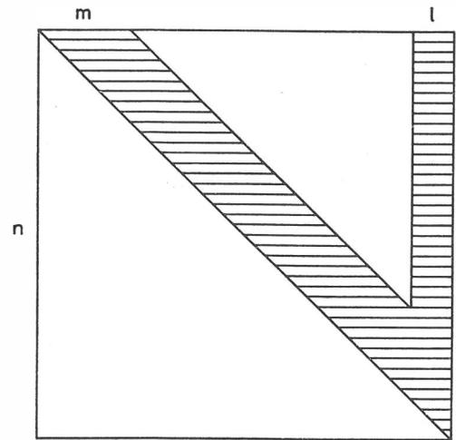
Fig. 1. Symmetric banded-bordered coefficient-matrix of reduced normal equations (elements below main-diagonal are suppressed)
