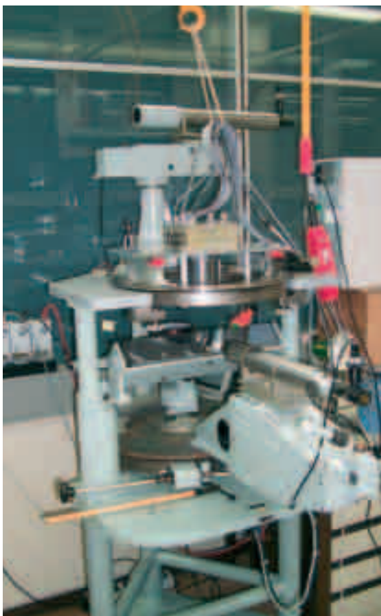
Figure 1. Goniometer calibration of individual DMC camera head at Zeiss (© Zeiss).
