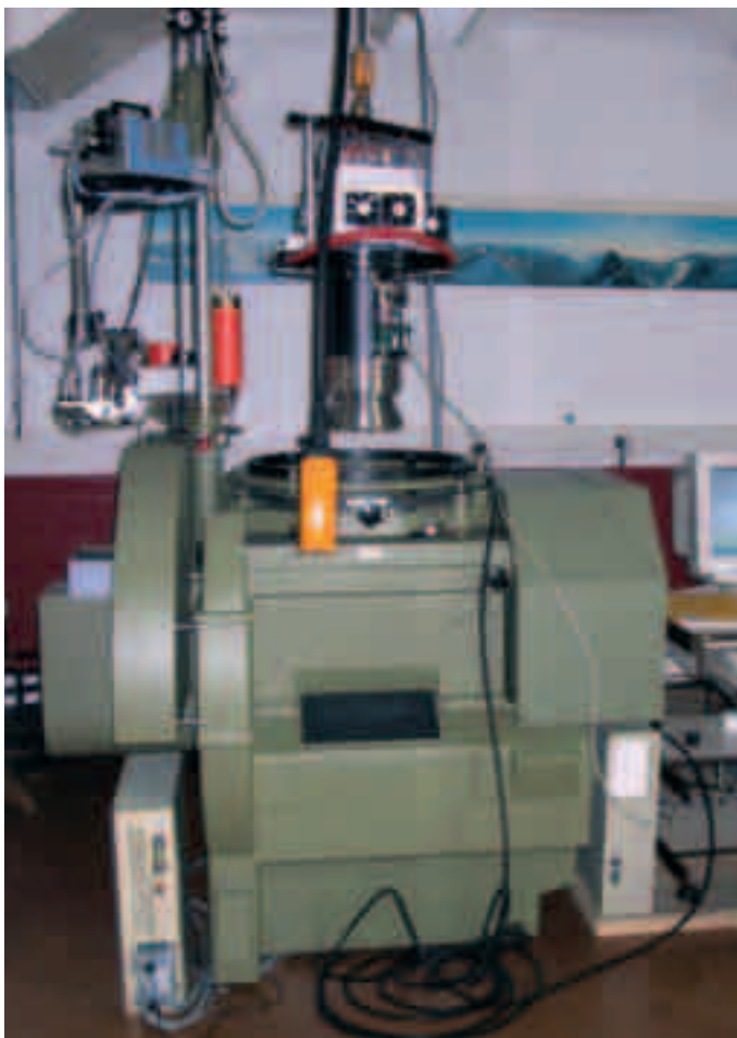
Figure 2. Goniometer calibration of ADS40 at Leica (© Leica).
