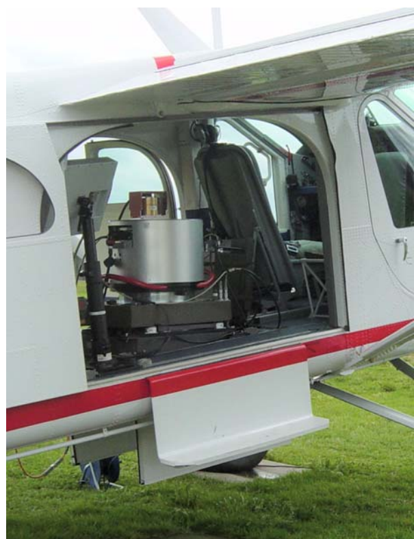
Figure 10, ADS40 aircraft installation for experimental test flight (© Leica)
