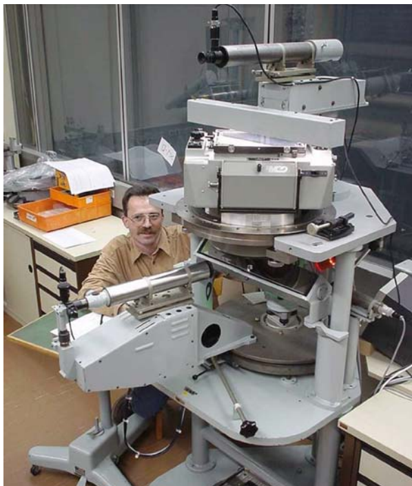
Figure 5, Zeiss goniometer calibration facility (© Zeiss)
