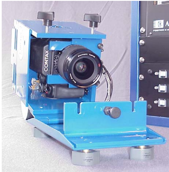
Figure 3, DSS medium format camera with proprietary exoskeleton for camera housing stabilization (© Applanix)
