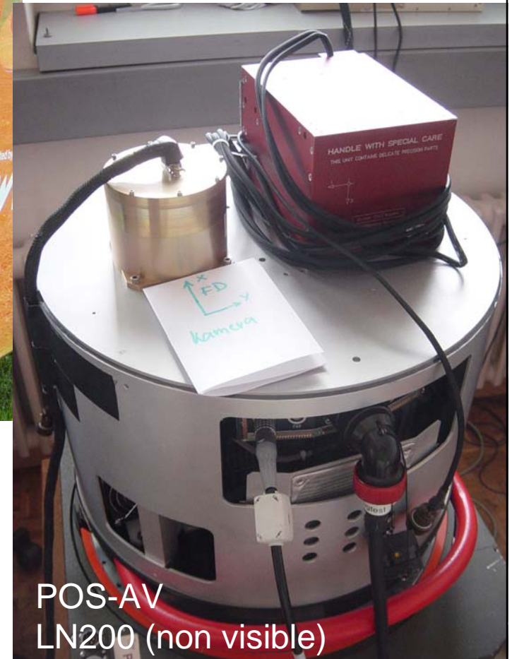
ADS camera head including different IMUs
