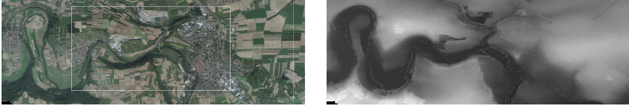
Figure 2: Ortho image (left) and DSM (right) of the UltraCam data set in 20 cm/pixel. The part that is covered in the data sets with 8 cm/pixel is marked by a white square.
