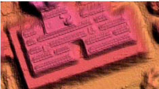
Figure 11: Example: UC-X, 8cm GSD DSM of a industrial building with solar panels on the roof.
