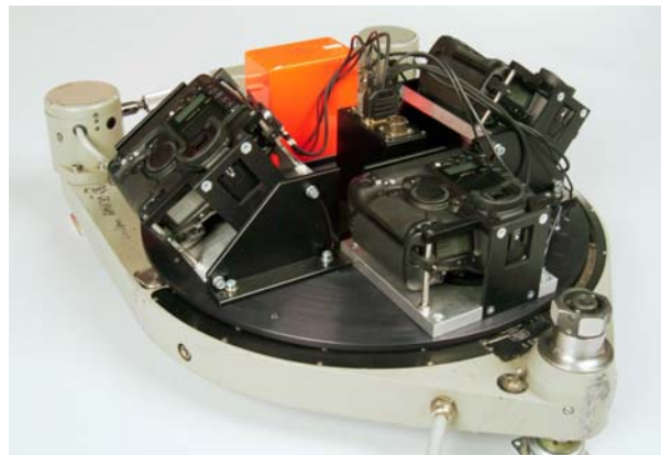
Fig 1 DLR 3K-camera system consisting of three Canon EOS 1Ds Mark II, integrated in a ZEISS aerial camera mount
