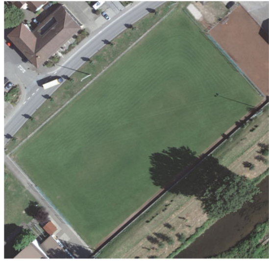
DMC image used for DSM generation, test site sports field (GSD 8cm)
