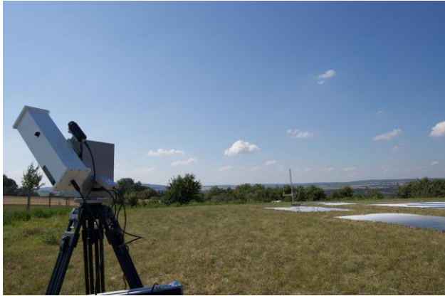
Fig. 6: Sun photometer on the test site at Vaihingen/Enz
