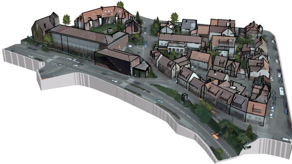
Fig. 1: 3D-aspect with stereoplotting results, Area 1 “Inner City”, UltraCamX, 8cm GSD.
