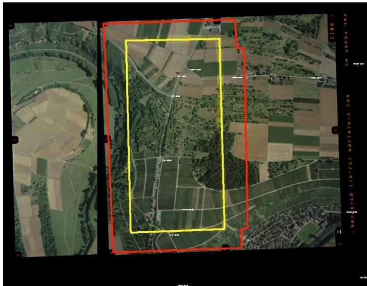
Fig. 12: Triply GCP re-measurements: Border lines of model area (yellow) and border area (red) for RMK, 8cm GSD images.
