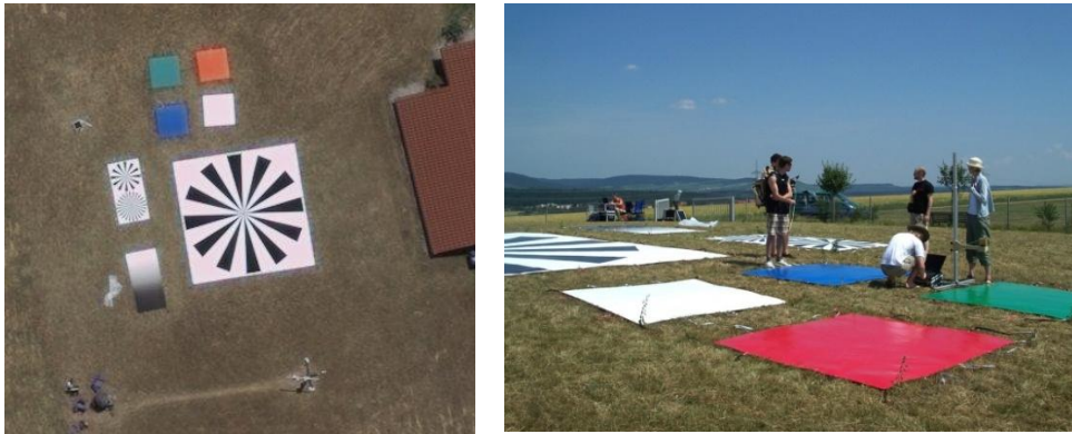
Fig. 2: Vaihingen/Enz radiometric test field from the air (left) and ground team members performing spectrometer measurements parallel to sensor flights (right).
