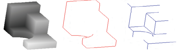
Figure 3: Curve block segmentation using different thresholds to detect step edges (red) and crease edges (blue).
